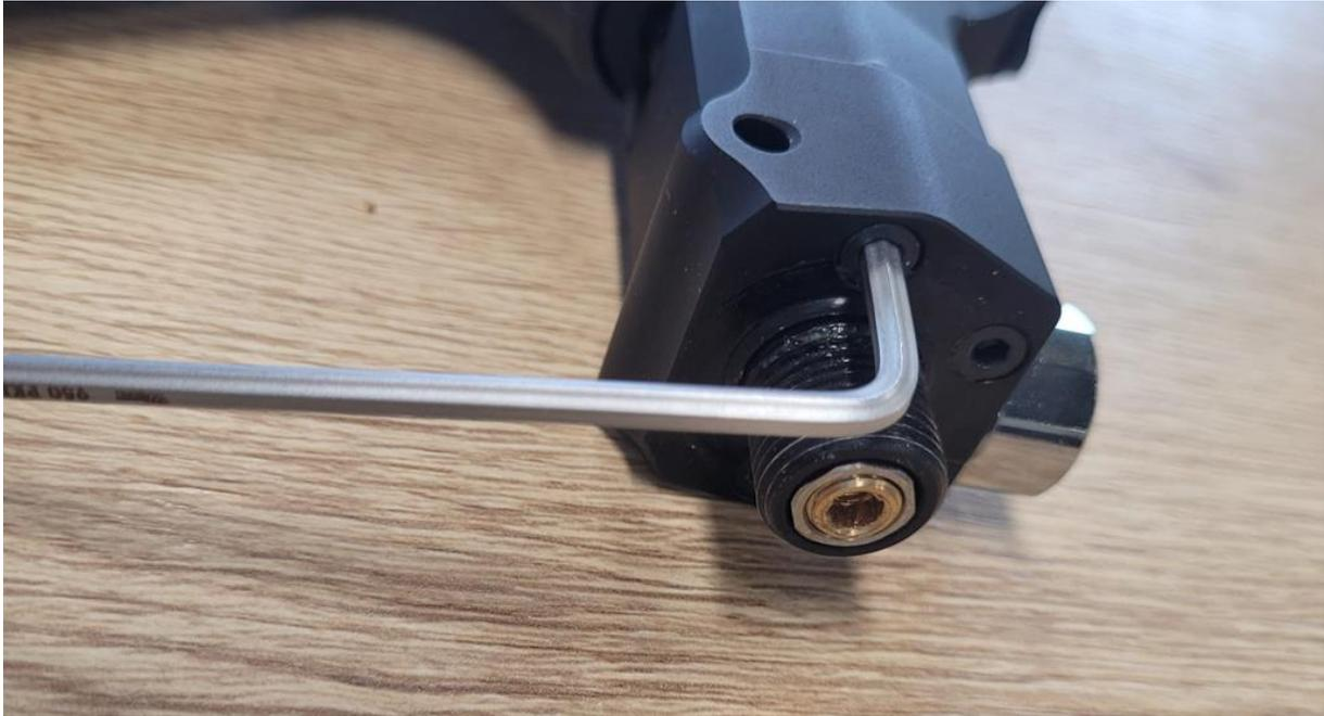
Unscrew the screws in steps using a 3mm allen key, and make note of the torque required to unscrew them to give you a feel how hard they need to be tightened afterwards. When unscrewing first undo all 3 only a little in a crosswise pattern. Repeat the steps until all 3 are loose.
