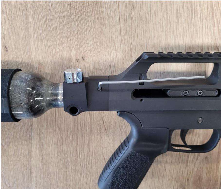
Drain the pressure tube so the rifle is totally empty by turning the above shown screw counter clockwise, using a 2mm hex key, until you hear it hissing. After it stops draining check the gauge to ensure it is completely empty. And maybe dryfire to make sure it is completely empty.
