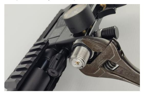
Now screw on the black bottle adapter and tighten it with a 24mm wrench or the adjustable wrench
