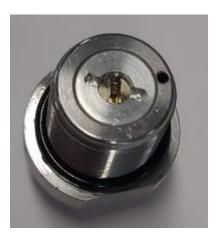
A 5 minutes turn counter clockwise will give a pressure increase of about 4-5 bar. Or ca 25-30 bar for ½ a turn
