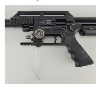
Unscrew the the 4 M3 screws using a 2,5mm hex key.
