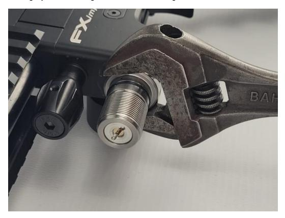
Lubricate the external oring on the regulator and the internal oring on the collar.
