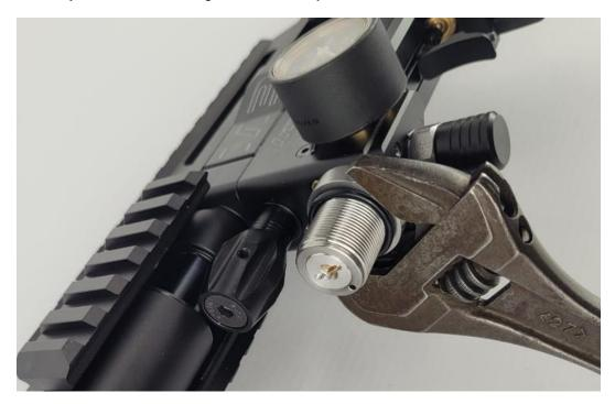
Next step is to plug the fill port hole with the supplied Blindplug.
