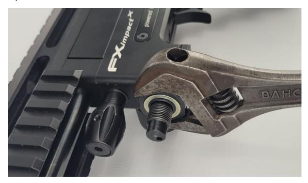
Now remove the fillvalve using the adjustable wrench or a 14mm spanned. You will be reusing the fillvalve.
