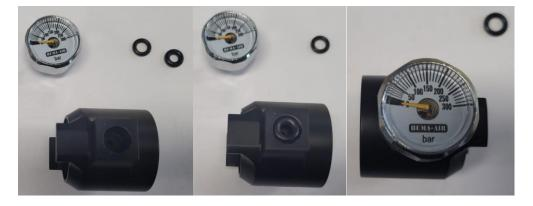
Here we opted to align it to have the gauge on the left side of the action. When alignment can't be made please swap the oring for the other one supplied.
