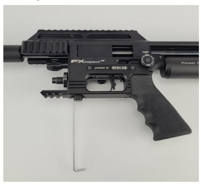
Unscrew the the 4 M3 screws using a 2,5mm hex key.
