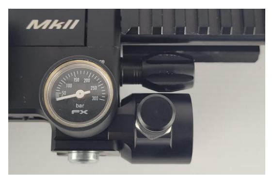
Last step is to screw in the bottle connector, ad some silicone to the small diameter to help seat the oring
