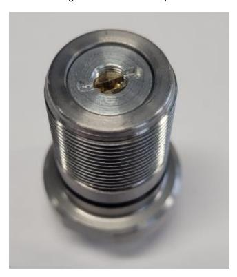
A 5 minutes turn counter clockwise will give a pressure increase of about 4-5 bar. Or ca 25- 30 bar for  $\frac{1}{2}$  a turn
