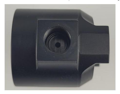
The fill valve can be screwn in and just tightened like it was on the gun. For the gauge choose one of the two orings supplied and screw in the gauge until it touched the oring then between  $\frac{1}{4}$  and  $\frac{1}{2}$  a turn further until it lines up with the bore of the collar.
