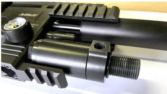
Now you can screw the bottle on the regulator body. Before you tighten the bottle, please align the regulator collar to the position you want it and after that, tighten the bottle firmly by hand.
