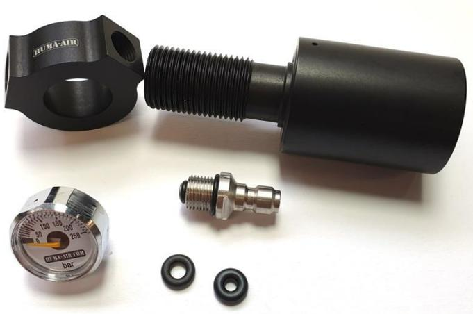
The foster male fill connector has a o-ring powered fill valve. By loosening or tightening the small screw you can adjust the fill speed.
