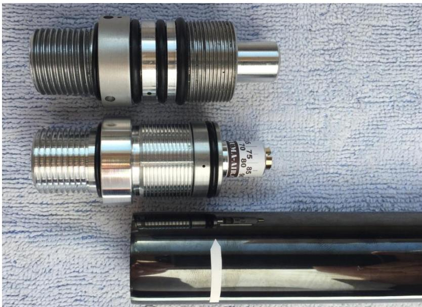
In the new regulator body you will find a tiny 1 mm hole. (see picture above) When you screw the pressure tube with the new regulator into action of the rifle, make sure this tiny hole points upwards to the breech. (You can temporarily mark the position of the hole on the outside of the regulator to check)
