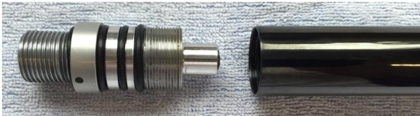
The position of front O-ring of the new Huma regulator is a few mm further inside the pressure tube compared to the original regulator.(see mark on the tube) Please check the surface of the inside of the tube where the o-ring will be seated, if it is smooth and without scratches. If not, please polish the surface of the tube until it is smooth. When finished clean the tube well and put a bit silicone grease inside the first 30-40 mm of the pressure tube.
