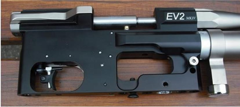
Unscrew the pressure tube from the action and after this, unscrew the original regulator from the pressure tube. It can be tight so a piece of rubber or leather belt can help you unscrew it without causing damage. After this, remove the pressure gauge assembly. In the action/regulatorbody there is the original valve return spring. Don't forget to place it back again!
