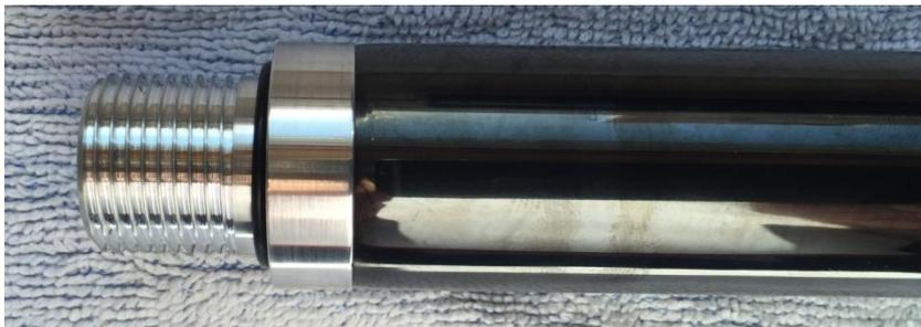
Now you can screw your pressure tube again to the action of the rifle. Check the marked position of the hole, and if it is ok you can pressurize the rifle.
