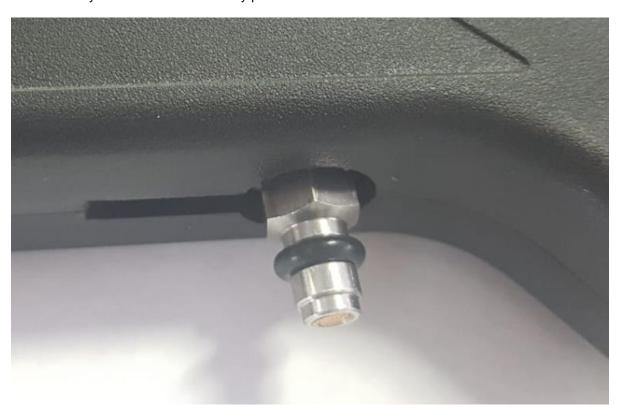
The o-ring slides into the groove in the foster coupler!
