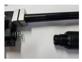
When unscrewing the cylinder from the action, most of the times the endplug will come out together with the cylinder.
