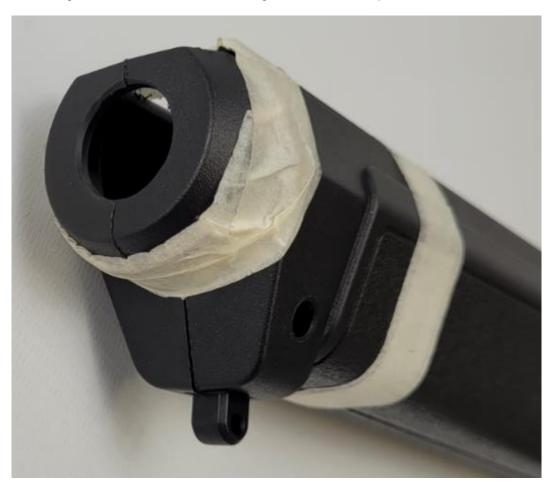
Using a stepped drill is easiest for creating a fitting hole, but a Dremel can also be used. We drilled the hole to approximately 21mm so the endplug piece has ample room to stick out of the stock.
