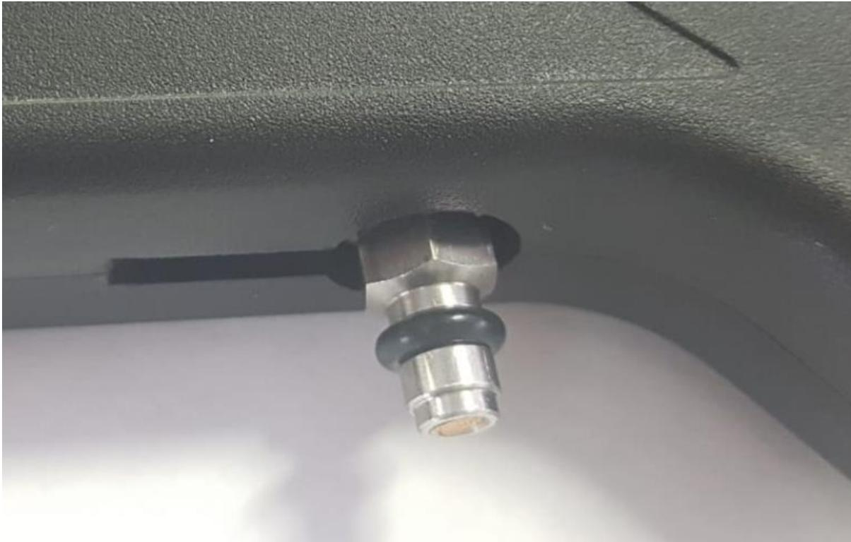
The o-ring slides into the groove in the foster coupler!
