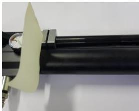
Now you can repressurize the system by using the new foster male connection on the front of the pressure tube and check for leaks.
