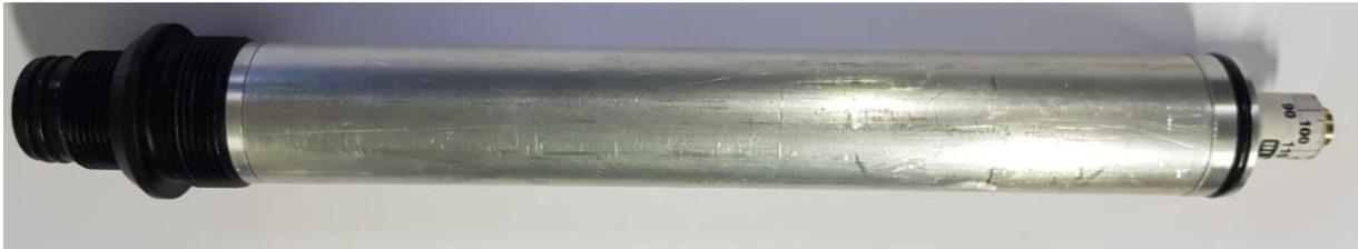
After lightly lubricating the o-rings on the regulator you can now slide in the regulator and screw the endplug back on the cylinder and the action but keep a very tiny crevice for reference pressure to easily let air pass past the endplug. Paper width will be sufficient (see picture below)
