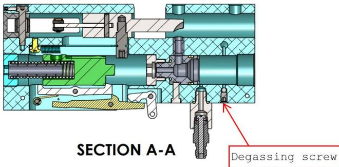
After depressurizing the rifle the air cylinder can be unscrewed from the action.
