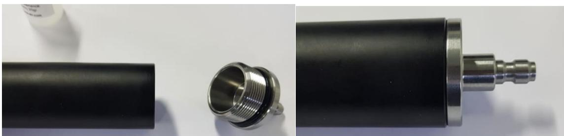
Then continue with removing the o-ring that seals the other endplug of the pressure tube. The o-rings on the regulator will take over that function and removing this o-ring will ensure the regulator can function properly. See picture below. Leave the o-rings on the action block connection just remove the large one on the cylinder side connection.
