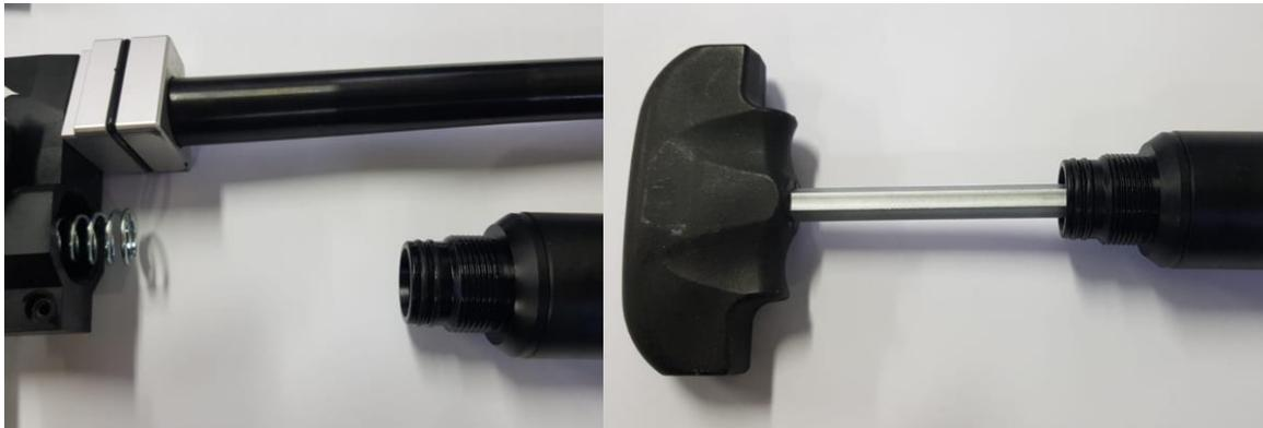
When unscrewing the cylinder from the action, most of the times the endplug will come out together with the cylinder. You can use a fitting hex wrench to unscrew the plug from the action.
