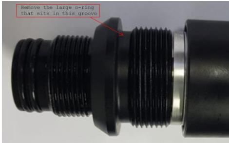
The endplug of the pressure tube goes onto the regulator adapter what is fitted to the long plenum tube of the regulator. Lightly lubricate the o-rings with silicone grease prior to assembling.
