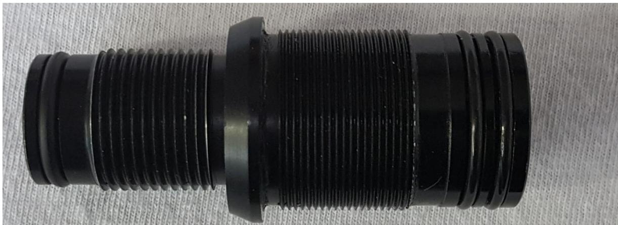
Remove the 2 o-rings that seal the adapter to the cylinder.
