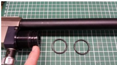
Now take your regulator and using a silicone grease. Grease the o-ring. Lightly grease the inside of the airtube where the reg will sit. This helps sliding in the regulator.
