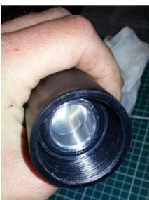
Slide the regulator in the tube being carefull not to damage the o-rings.The regulator has a tiny breathole, please assemble the regbody with this hole facing upwards to the breech.
