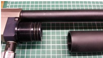
Remove the 2 o-rings that seal the action to the cylinder.
