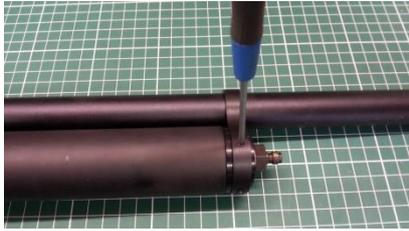
Loosen the 3 setscrews that hold the barrelband to the cylinder. Once these are loose you can slide the barrelband forward.
