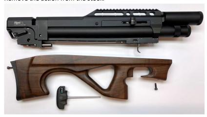
Unscrew the allen bolt on the side totally untill the end
