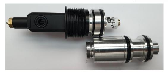
Now push the dummy plenum inside the pressure tube using some silicone grease and screw the valve house with regulator back inside the pressure tube. Do not forget to close the de-pressurize screw again.
