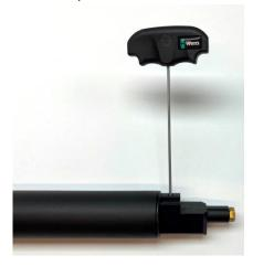
Then unscrew the valve from the pressure tube and make sure you remove the factory regulator from the pressure tube as it sometimes unscrews itself inside the pressure tube.
