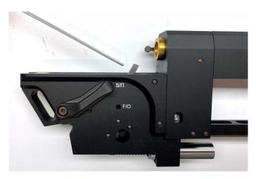
No you can easily remove the hammerspring and guide pen and replace the stronger hammer spring for the new weaker spring.
