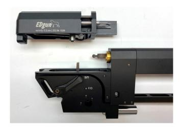
The next step is to tap out the F/O pen using the pendriver. The F/O pen blocks the hammer stroke length and the hammer needs to go further forwards to remove the hammerspring.
