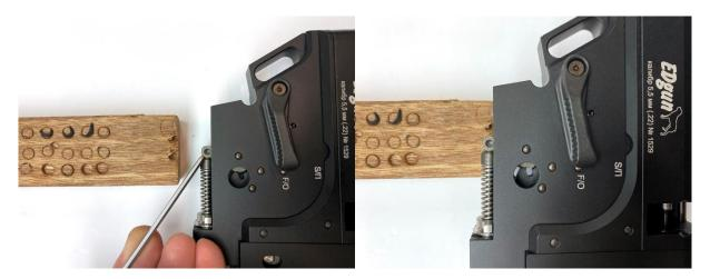
As the hammer is blocked in it stroke length we need to remove the breech. The breech is hold by just 1 screw on the back. Unscrew it and pull it straight back. You can easy help it by cocking the rifle and pulling the breech backwards simultaneously. A video how to do it can be found here <a href="https://youtu.be/ev0nPyLA\_Qw">https://youtu.be/ev0nPyLA\_Qw</a>
