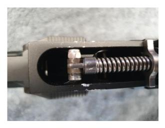
After placing the new hammerspring you can assemble the rifle back again. Following the same steps. and when ready you can fill your rifle and start testing and adjusting the hammerspring using a chrony to get the perfect pelletspeed.
