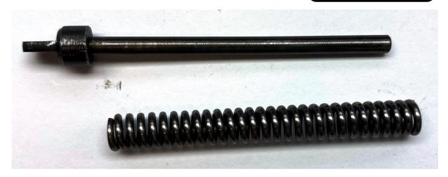
After fitting the new hammerspring you can replace the F/O pen again and make sure the hammer is upwards position before the pen is fixated. Then place the small the small trigger pen again. (when it gives you trouble getting it in again you can replace it by a allen bolt M3x10 mm with a nyloc nut)
