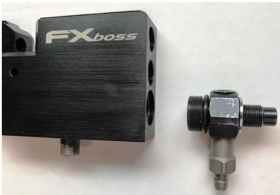
Pull the factory reg out of the chamber using some pliers
