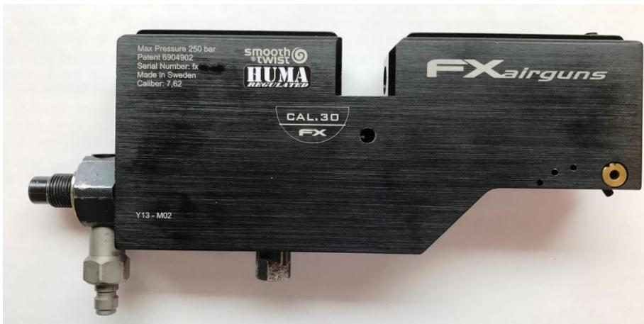
Please check if the adapter does not touches the setscrew when it is screwed in again by measuring the length. (If it does, the reg needs to be pushed into the rifle some more OR open up the hole in the bottle adapter for about 2-3 mm in length and 8 mm diameter, but this is very unlikely)
