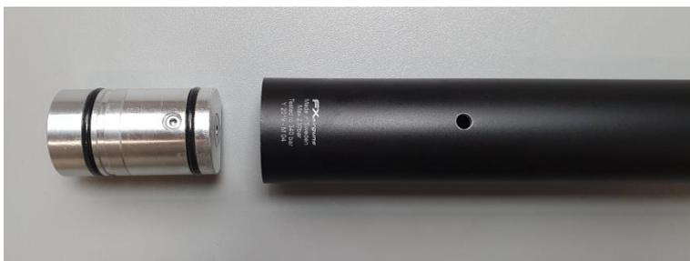
Now take the Huma-Air power tune regulator set and check if the regulator is fully clean and free of dirt. If not, clean it and apply some silicone grease on the walls of the pressure tube. Then slide the new regulator into the pressure tube, facing the label side to the barrel end.
