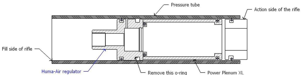
After this screw the pressure tube on the action and you can assemble the rifle back again.
