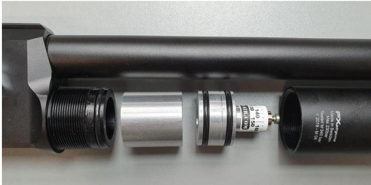
Now slide in the Huma-Air aluminum spacer, this will hold the reg in the correct position in the tube. This additional spacer of plenum will add about 14 CC of regulated air to your rifle!
