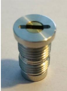
Just like the factory regulator the Huma regulator can be turned up in pressure while under pressure. **But you cannot decrease the regulator pressure while the rifle is pressurized. It will ruin your valve disk immediately.**
