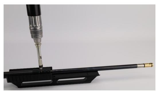
Now the complete assembly is slid back and the 3 top screws as well as the barrel securing screw in the rear action black needs to be tightened.
