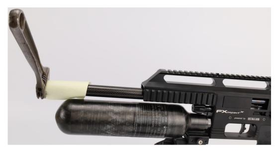
Possible issues you might encounter with assembling the kit are mostly related to the carbon fiber, although we strive to have the carbon sleeve produced as close to spec as possible. Due to the resin coating involved in producing these and tolerances on the FX STX barrel it could be that the carbon needs to be sanded ever so slightly.
