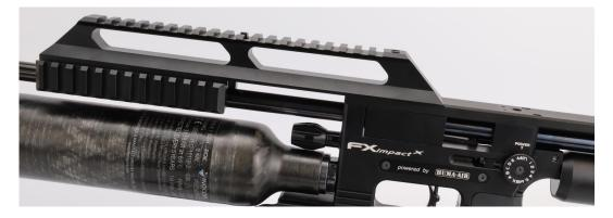
Once properly aligned you should be able to slide it home easily. Then using the supplied M3x30 and M5x25 screws, secure the extended rail to the impact guiding plate. For this use a 2,5mm and a 4mm hex key. No need to torque them down hard yet as it will be removed later on.
