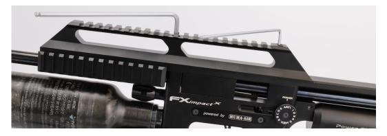
Now use a torque wrench to set the 6x M3 screws to the right torque. Torque on the 6x M3 screws should be between 1.75-2Nm (±15-17.5 Inch.lbs). As you can see here the barrel and rail will form a rigid assembly. If you have barrels and scopes to spare, you can also pair a scope to your barrel rail assembly for the least amount of sight in required.
