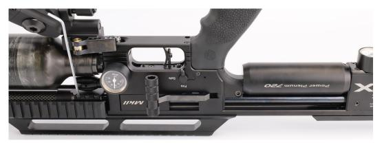
Now unscrew the barrel securing grub screw from the rear action block using a 4mm hex key and unscrew the 3 screws from the rail again. After this is done the complete assembly of rail and barrel can be pulled out to the front.
