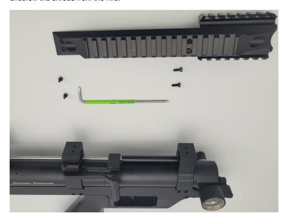
Unscrew the cheeckpiece from the back of the action using 3mm hex key
