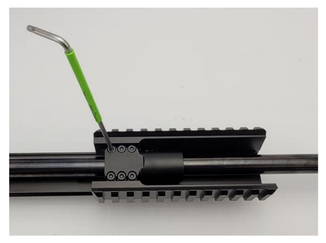
After that use a torque wrench to set the 6x M3 screws to the right torque. Torque on the 6x M3 screws should be between 1.75-2Nm (±15-17.5 Inch.lbs). As you can see here the barrel and rail will form a rigid assembly. If you have barrels and scopes to spare, you can also pair a scope to your barrel rail assembly for the least amount of sight in required.
