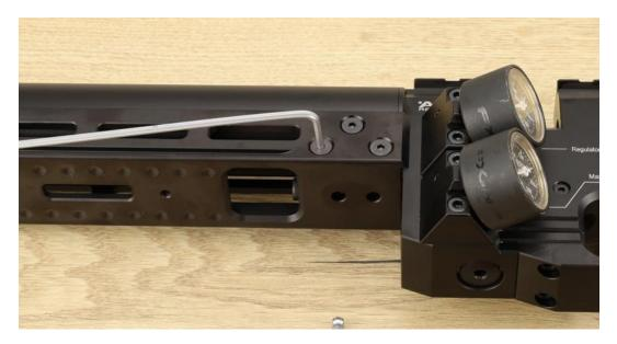
After these have been removed you can slide of the complete rail assembly from the front.
