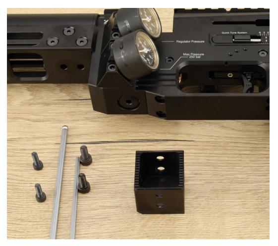
Now remove the 6 M4 countersunk screws on either side of the rail using a 2,5mm hexkey
