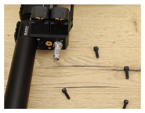
Tightly secure the adapter using a 15mm hexwrench
