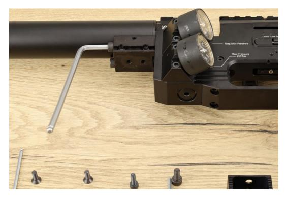
This will now reveal 2 brass plugs. Remove the bottom one from the Dynamic Block. Check if the oring is in good condition.
