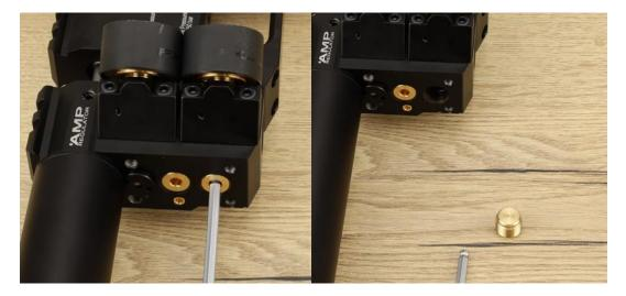
Screw in the bottle adapter in the hole. Use a little silicone grease on the nose of the adapter to help seat the oring again.
