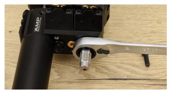
Put a small dab of antiseize on the cylindrical part of the adapter where our support plate will slide onto.
