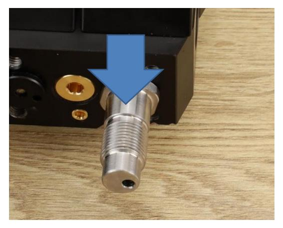
Now you can slide the support plate over the adapter and screw in the supplied M4 and M5 screws with 3mm and 4mm hexkey accordingly.
