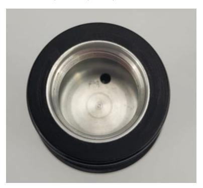
To this part place an air blower pistol used on your shop compressor and place a piece of tissue in the regulator orifice then cover it tightly with your hand. And then apply pressure.
