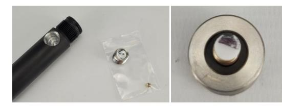
Unscrew the piston subassembly from the locknut so you can start assembling the parts together. They are temporarily assembled by us to protect them during transport. Most times the valvedisc will stick to the piston as can be seen in the picture. But if it falls off be sure to assemble it in the same orientatie as it was as delivered.
