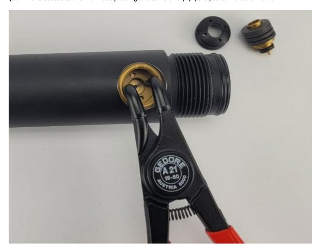
Once removed you'll see the sealing bushing and the ceramic ball underneath it.
