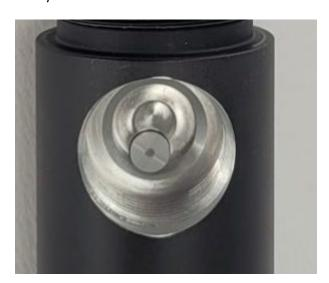
Now carefully clean the regulator orifice and lucricate it with some silicone grease
