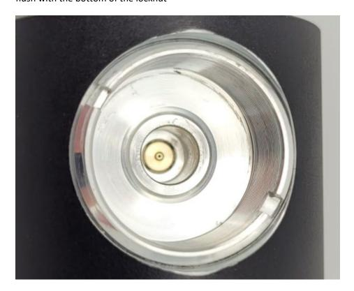
Insert the valvedisc in the bore or when it is still on the piston you can commence to screw in the complete subassembly.
