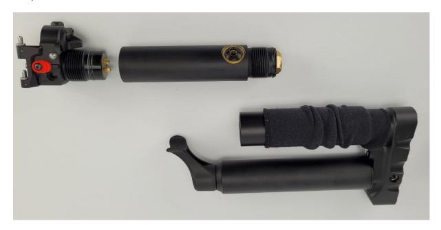
To prepare the EAR plenum body for it's new internals you need to remove all the old Edgun EAR regulator parts.
