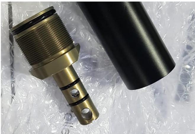
Make sure the valve body and threads are clean and free of grease and oil,
