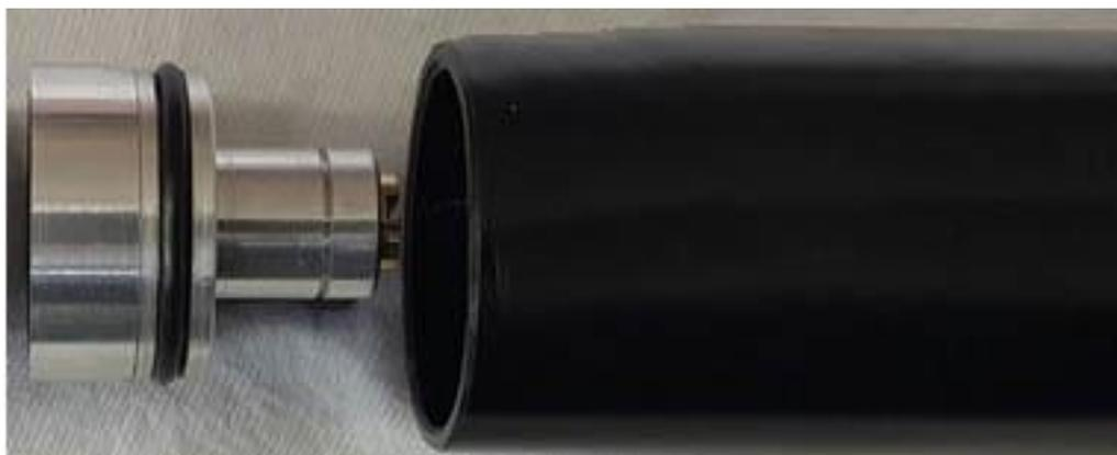
Make sure the tiny breath-hole of the regulator body is facing upwards to the breech when the tube is screwed on.
