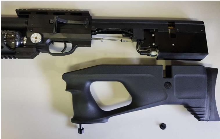
Drain the pressure tube so the rifle is totally empty by, for example, dry firing
