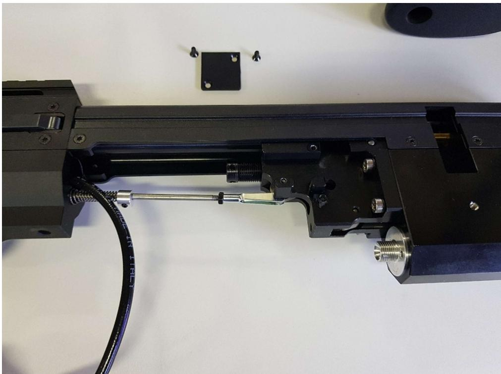
Behind the cap you just removed you see the factory regulator. Using a long M4 screw it is easily pulled out.
