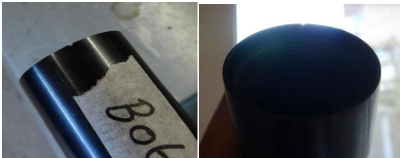
Following your mark on the valve body, file a small groove in the longitudinal direction of the screw-thread of the valve body.
