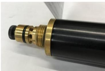
Slowly fill the pressure tube and check for leaks,
