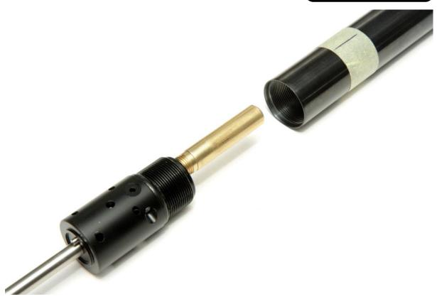
To allow regulator fitment the brass exhaust valve "pot" or "plenum" requires removal. It's a push fit onto the valve spring retainer and is assembled with retaining compound. Ideally this needs to be heated moderately with a torch or heat gun to allow it to be gently wiggled, twisted and pulled off using padded pliers or a gloved hand.
