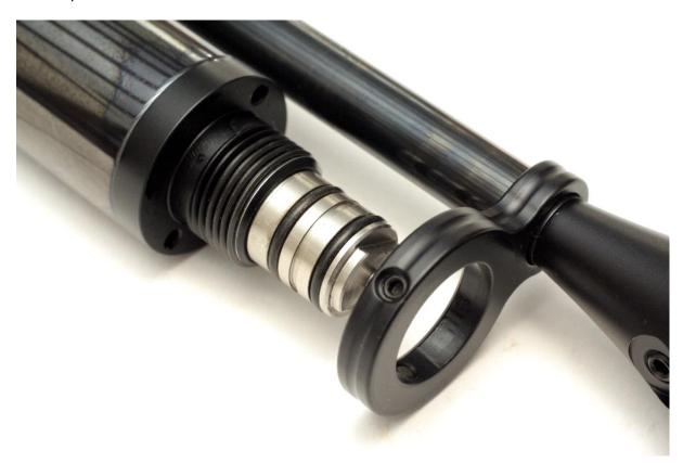
If working on an S410, remove the magazine indexing assembly by fully unscrewing the three retaining bolts using a 2.5mm Allen key, and removing the assembly en-block from the loading bolt housing.
