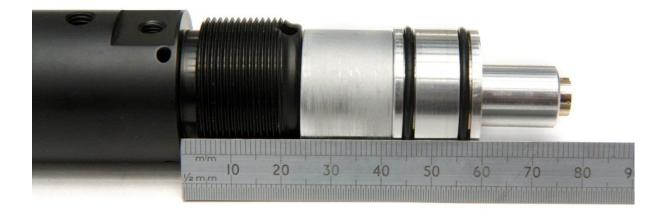
Since dimensions can change with revisions in component design, arrange the exhaust valve housing, standoff and regulator together as illustrated above and measure the distance from the cylinder mating face on the exhaust valve housing to the mid-point between the two O-rings on the regulator to check this value for yourself.
