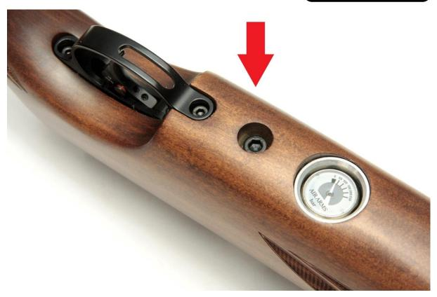
Next, remove the fill valve cover if still fitted and using a 2mm Allen key, slacken off the two grub screws on the barrel support and pull it forwards on the barrel, over the end of the filler valve assembly.
