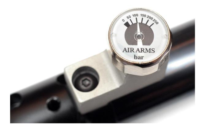
It's usual for this to creep up slightly during the first few minutes of pressurisation as the regulator "settles". In the unlikely event that pressure continues to climb until the rifle's pressure gauge is displaying a value close to the 150bar in the cylinder, there is a leak either within the regulator or at the O-rings around its circumference (the latter case only being possible if there's no breather hole in the cylinder).
