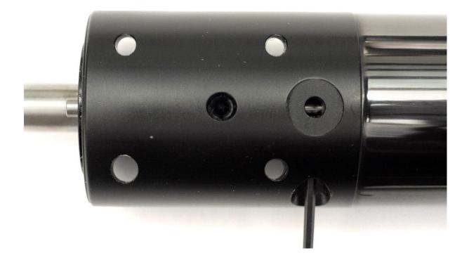
Next, re-fit the striker and spring to the guide rail on the rear of the exhaust valve housing, then add the spring seat to the rear of the striker spring and fit the striker housing over the whole assembly. The guide rail should be thoroughly cleaned before re-assembly, but not lubricated since the striker runs on self-lubricating bushes.
