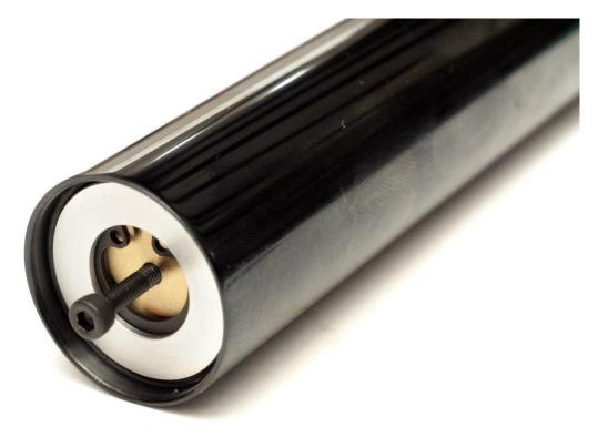
Alternatively it's possible to de-pressurise the rifle, remove the barrel support and inlet valve
