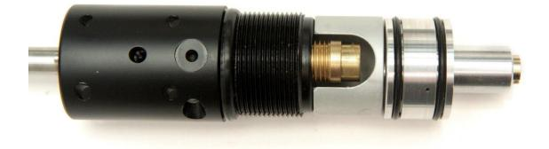
Screw the cylinder onto the exhaust valve housing – if excessive tightness is felt back off any try again, if it persists separate the two parts and push the regulator a little further into the cylinder.
