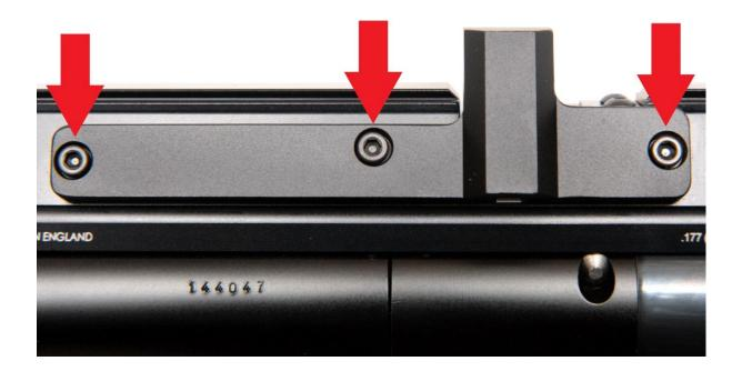
Lay the action on its top and remove the six loading bolt housing retaining bolts in the underside of the action, working front to back and keeping your finger and thumb between the barrel and cylinder to prevent contact. Note that on current rifles these bolts are different sizes and will require both 2.5 and 3.0mm Allen keys.
