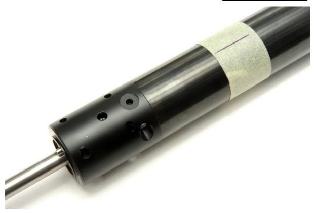
Unscrew the air cylinder from the exhaust valve housing – this is easier on some guns than others, but can usually be done by hand. If the cylinder proves difficult to remove I supply a collet tool for gripping the cylinder, which is available on my website [LINK]. In extreme cases heat from a hot air gun or gas torch can be useful in shifting particularly stubborn cylinders.
