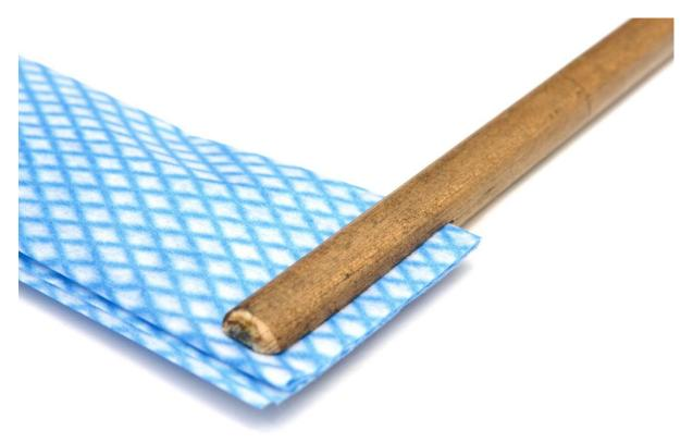
240-400 grit Wet and dry paper is the abrasive of choice and can be used dry, or preferably with a lubricant such as oil, paraffin or water. If using water be sure to thoroughly dry and re-oil the cylinder when finished.
