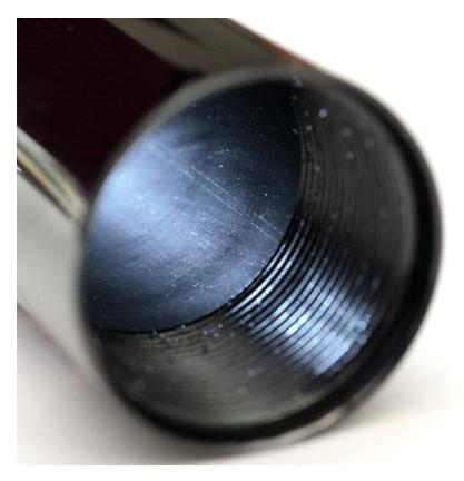
It's possible for small surface imperfections on the inside of the cylinder to cause very slow leaks; allowing air to bleed past the external seals and escape from the breather hole in the cylinder.
