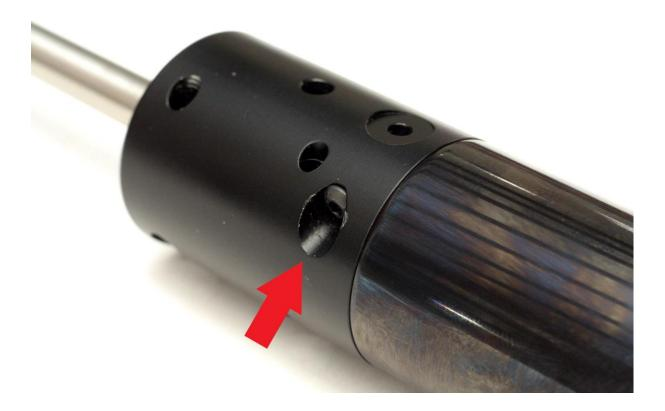
Looking at the transfer port itself in the exhaust valve housing from above, you'll notice the conicalend of the port adjustor screw projecting into the port.
