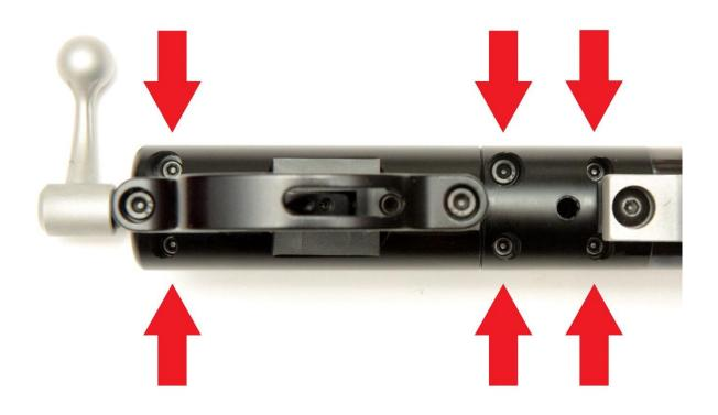
Holding the action vertically with its rear uppermost, unscrew the single bolt at the rear of the striker housing using a 5mm Allen key and lift the striker housing away from the exhaust valve assembly. Slide the striker off of its guide rail at the rear of the exhaust valve assembly along with the striker spring and its seat.
