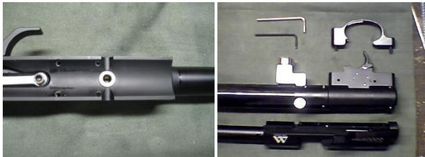
Remove the Power Adjustment knob by loosening the set screw in the valve body directly under the knob. Taking this knob out is not required, but it will make removing the cylinder easier. There is a small spring and a dowel pin under the set screw. Place them aside so they are not lost.
