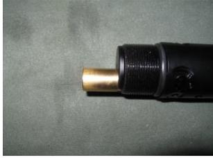
This is what the spacer should look like when placed around the shortened POT. Notice the internal shoulder inside the POT that retains the valve spring. Also notice the chamfered inside edge of the POT.
