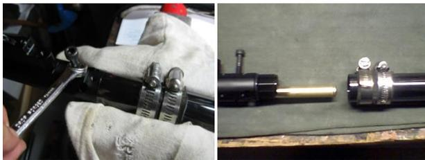
Mark the POT with the length of the spacer provided with the regulator. This is the maximum length the POT could be and still allow proper installation of the regulator. The POT actually will be cut a bit shorter than this length. Remove the POT by loosening the set screw in the side of the Valve Body, just where the POT is attached.
