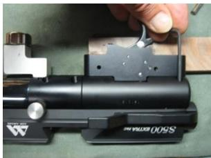
The Breech and Barrel assembly can now be lifted from the rest of the rifle body. Be careful not to lose the white plastic seal washer, it can fall off easily.
