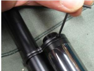
Remove the two screws from the end of the Striker Body. (Note this is a S500 FAC assembly and does not have anti-tamper devices plugging the screw holes. If your model is not FAC, the plugs will need to be removed.) Remove the four screws from the Valve Body in front of the trigger. These screws will be easier to remove if the trigger guard is removed first.
