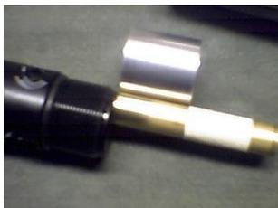
To get the correct placement of the breather hole for the regulator in the cylinder, place the spacer and regulator at the end of the valve body. Measure the distance from the face of the valve body to the breather hole in the regulator.
