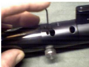
Remove the Cylinder Pressure Gauge. This is a very tightly torqued screw, so be careful not to strip the hex. It will come out and there is no thread locking compound used here, it is just very tight. Again, removal of the pressure gauge is not required, but it will make removing the cylinder easier.
