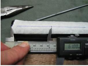
Carefully center punch and drill the breather hole using a 1mm or 1/16 inch drill bit. This is best done in a drill press with the cylinder firmly clamped in place, but if you are careful not to let the bit wander, it can be done with a hand drill.
