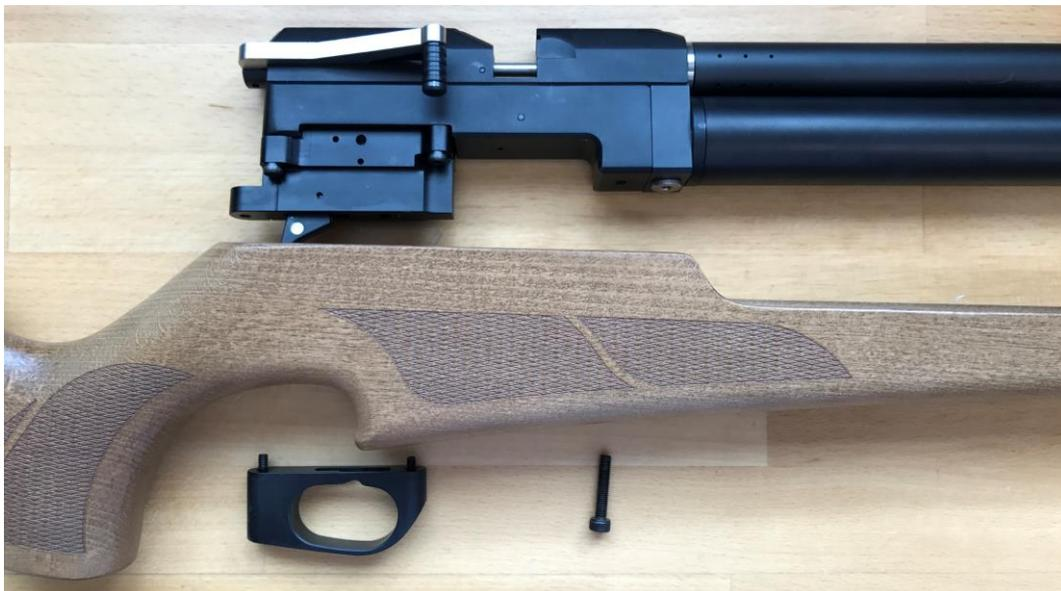
2. Remove the barrel, barrelshroud by loosening the grub screws in the breech.
