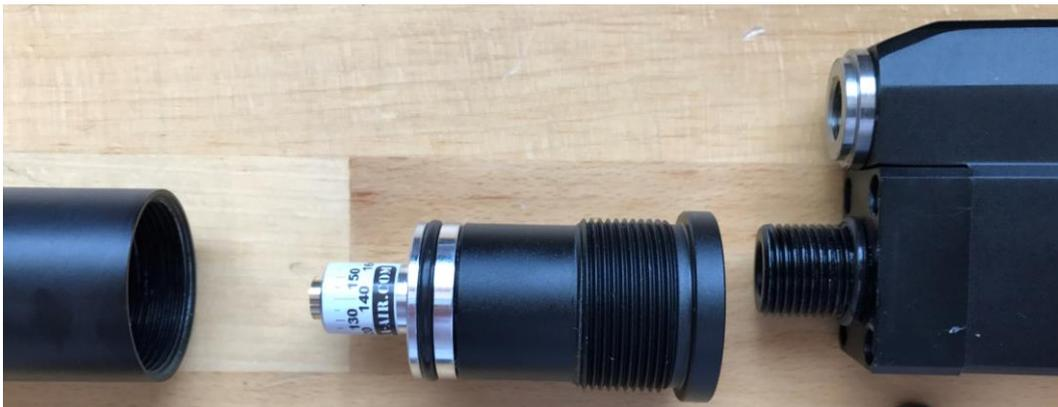
5. Now you can screw the endcap into the pressure tube again and screw them back on to the action. Before you pressurize the tube again, please unscrew the pressure tube and the endcap just about a  $\frac{1}{4}$  to a half turn open, so there is a tiny gap (max 0,5-1 mm) between the pressure tube and the pressure tube endcap. This allows the regulator to breathe to the atmosphere better.
