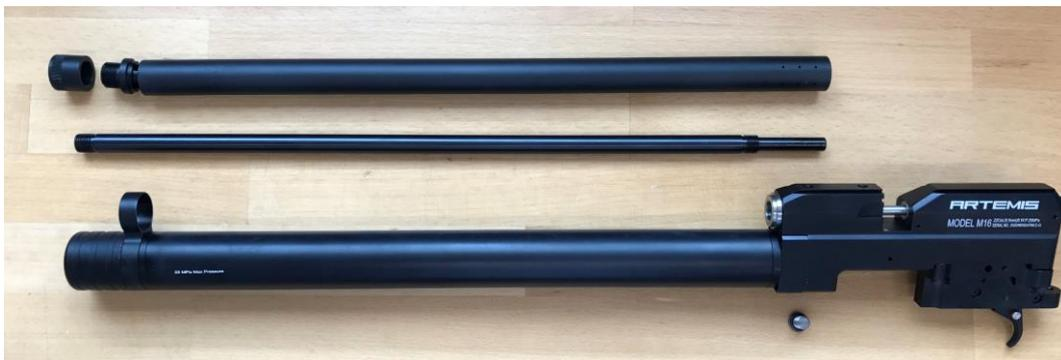
3. Unscrew the pressure tube from the action. Sometimes the regulator adapter is still inside the pressure tube, then loosen it separately as in the picture below.
