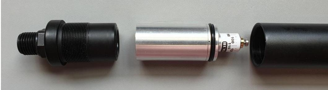
11. Now you can screw the endcap into the pressure tube again. Before you pressurize the tube again, please unscrew the pressure tube just about a  $\frac{1}{4}$  to a half turn open, so there is a tiny gap (max 0,5-1 mm) between the pressure tube and the pressure tube endcap. This allows the regulator to breathe to the atmosphere
