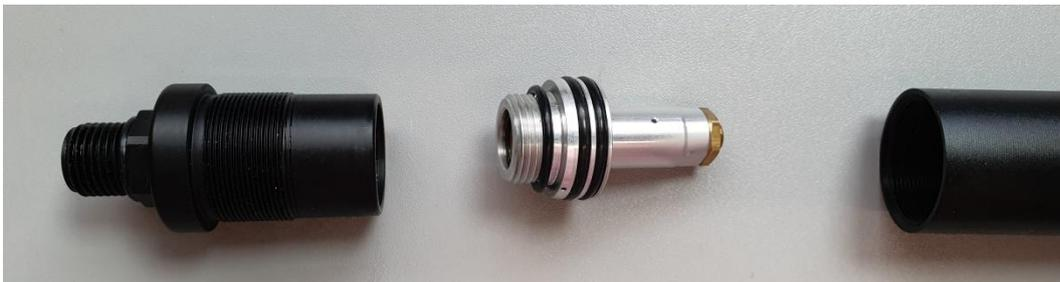
8. Now there are 2 options. When you have bought a Huma-Air tuning regulator as replacement for the Chinese factory reg or you have the Power Tune regulator with a treaded XL plenum (2021 model), you can now replace it the same way as the factory regulator was screwed in. Use some silicone grease to lube the inner wall of the pressure tube and o-rings
