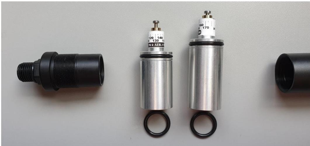
9. Place the large o-ring what is included with the regulator inside the endcap of the rifle
