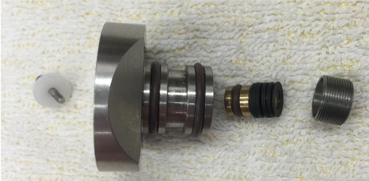
If you have unscrewed the factory regulator housing from the action, you can now place it back again and tighten it with the 4 bolts. Please place all original regulator parts back, except the valvestem what holds the white disk.
