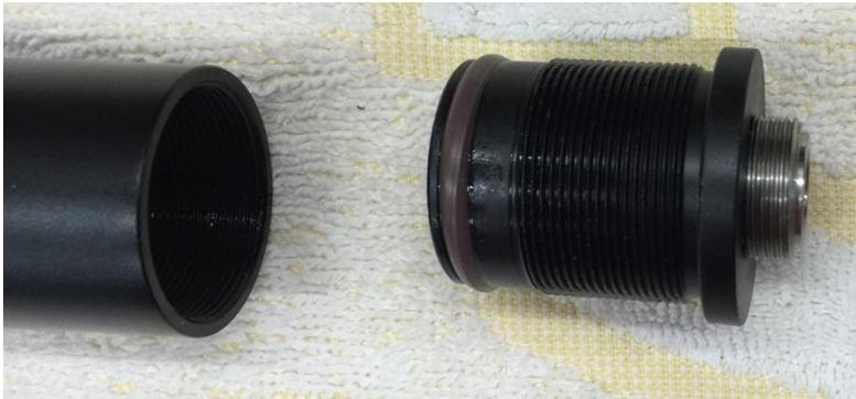
8. Now you can push the new regulator into the pressure tube. The scale label needs to be pointed towards the fill side of the pressure tube and the biggest diameter of the regulator will stand on the pressure tube's endcap. Because the o-ring of the endcap is removed, the regulator can "breathe" by the treads of the tube.
