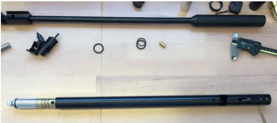
Place the transfer port what you have opened up in diameter to 4-4,2 mm back in it's place. Place all three screws back in their place and turn them in. **Tighten them AFTER you have assembled the breech in the right position.**
