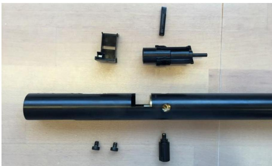
With an allen key or a piece of wood you can easily unscrew the fillcap from the pressure tube.
