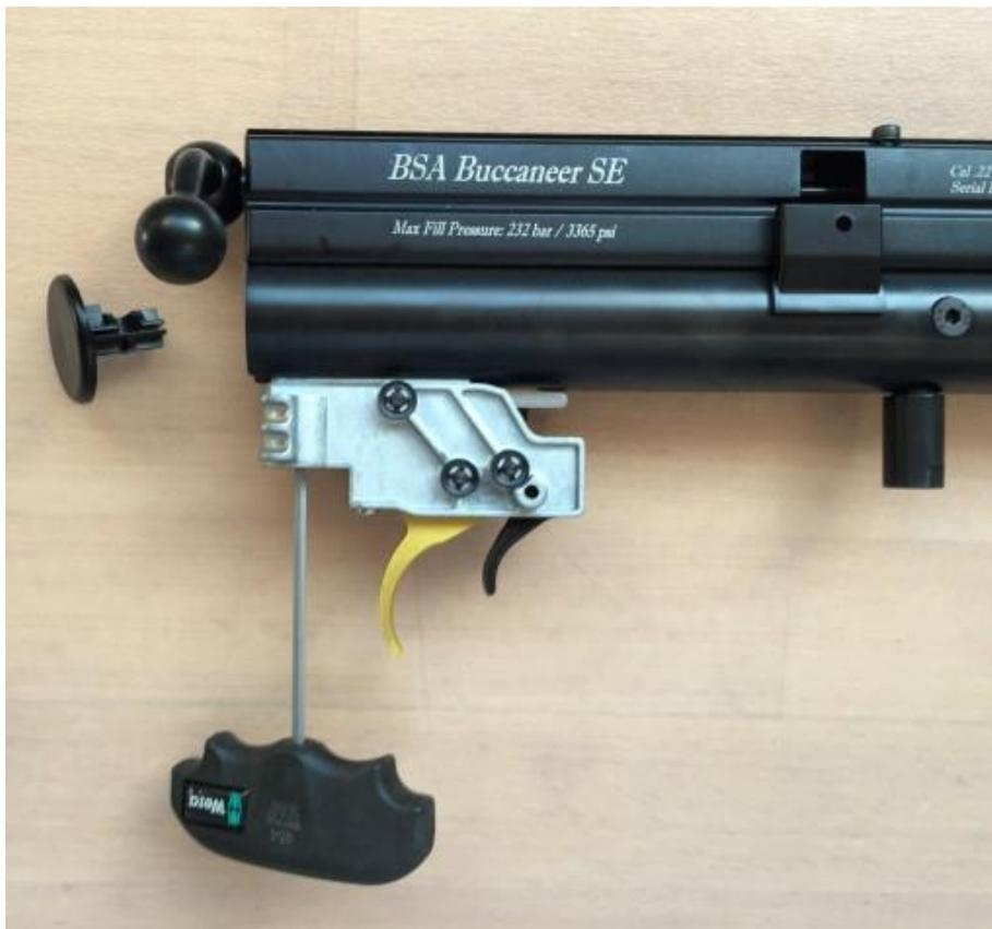
Below you see the transferport, You can take it out and open the inner diameter to 4-4,2 mm
