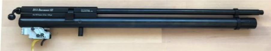
Remove fillcap and unscrew the barrelband
