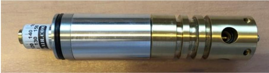
Now push the regulator-valvehouse combination into the pressure tube from the fill side. (do not try to push it in from the trigger-side, the slots in the pressure tube will damage your orings for sure)
