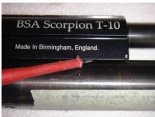
Turn off the pressure tube, pressure gauge assembly and finally the last piece of the tube where the valve house is inside. You can leave the pressure gauge itself in the assembly!
