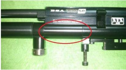
Loosen both the breech screws a bit so there is a bit space between pressure tube and breech. This prevents scratches on the tube when turning it loose. (you may also remove breech totally)
