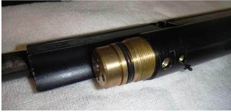
Unscrew the endcap of the valve house and take out the restrictor.
