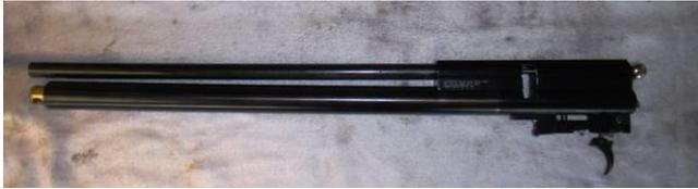
Loosen both the breech screws a bit so there is a bit space between pressure tube and breech. This prevents scratches on the tube when turning it loose.(you may also remove breech totally)
