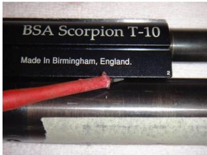
Turn off the pressure tube. If it's tight there could be pressure inside! Double check this.
