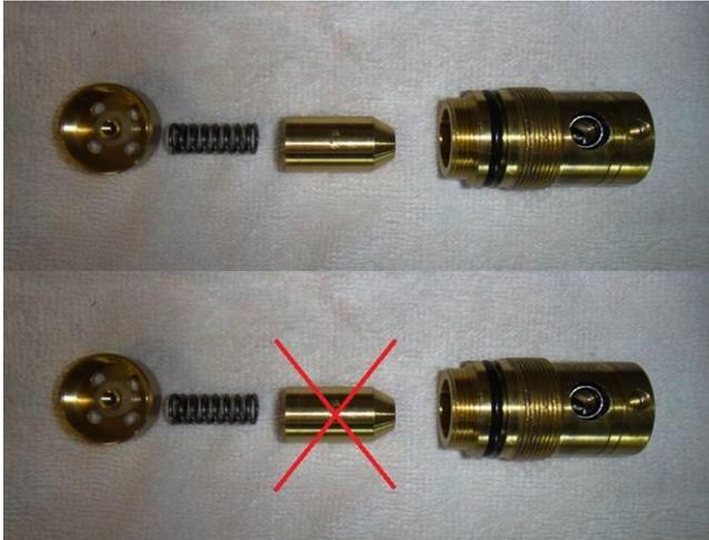
Remove the restrictor and screw the valvehouse back together
