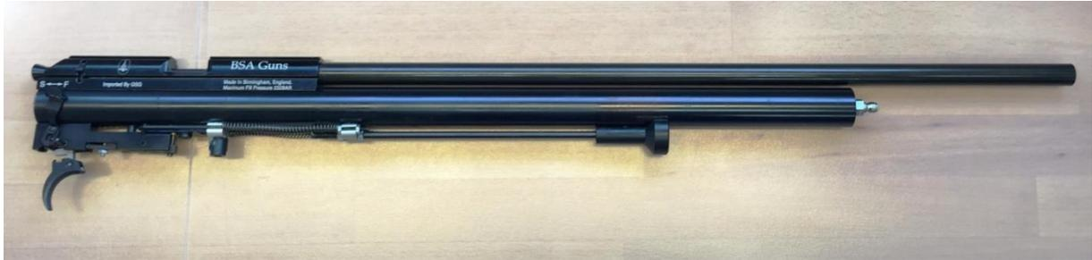
Loosen both the breech screws a bit so there is a bit space between pressure tube and breech. This prevents scratches on the tube when turning it loose.
