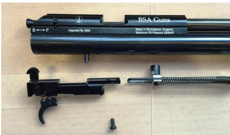
Turn off the pressure tube. If it's tight there could be pressure inside! Double check this.
