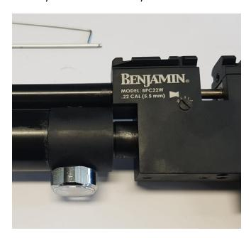
6. Now unscrew the gauge connector from the tube, and remove the orings from that. The cap (you see it in the middle is no longer needed, keep it safe if you plan to, later on, remove the regulator
