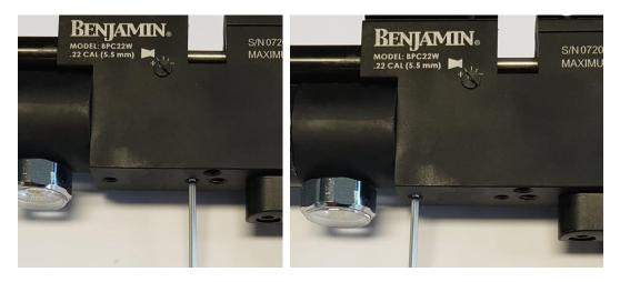
4.Loosen the grub screws from the barrel band and rotate the barrelband out of the way.
