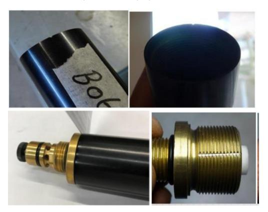
8. Now it's time to slide in the regulator. Don't forget to set it to your desired pressure before inserting it. Also use some silicone lubricant to keep orings sliding freely and keep the souple. Be sure the oring in the plenum face that is going to seal against the gauge connector is seated correctly.
