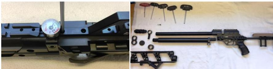
Unscrew the valve block from the pressure tube. This can be a tight fit, boiling water can help. Please remove the pressure gauge before doing this.
