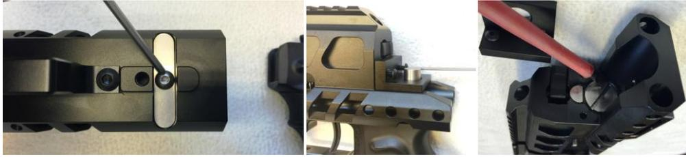
*If you notice power spikes every few shots it means that the regulator is not venting/breathing enough/properly. Check that the threads of the pressure tube and valve body are clean and free of grease, also make sure the valve block is not screwed too tightly into the air cylinder.*
