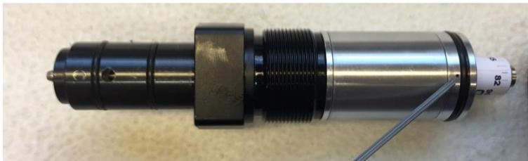
Screw the pressure tube together again and leave a tiny gap (0,5 mm) open between valveblock and pressure tube so the regulator can breathe.
