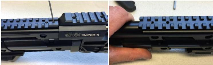
Unscrew the endcap of the fill-side and unscrew the allen bolt from the underside of the barrelband. Then carefully remove the barrelband by sliding it off. And also slide off the hand-grips.
