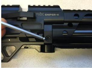
Unscrew both m4 allen screws on top of the rifle, inside the weaver rail. One is near the end of the barrel, the other is near the breech.
