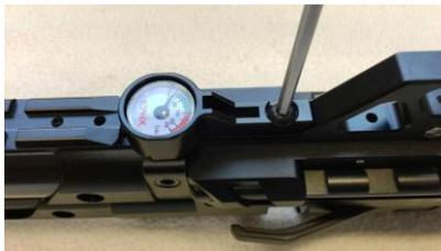
After removing the protection cap, two allen screws are visible. Please remove those and you can gently pull out the pressure tube.
