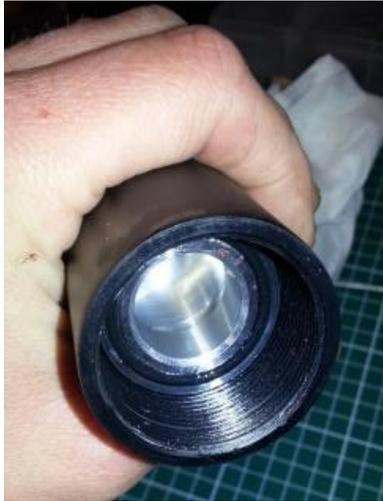
After this you can screw the endcap back on and pressurize your cylinder to check for any possible leaks.
