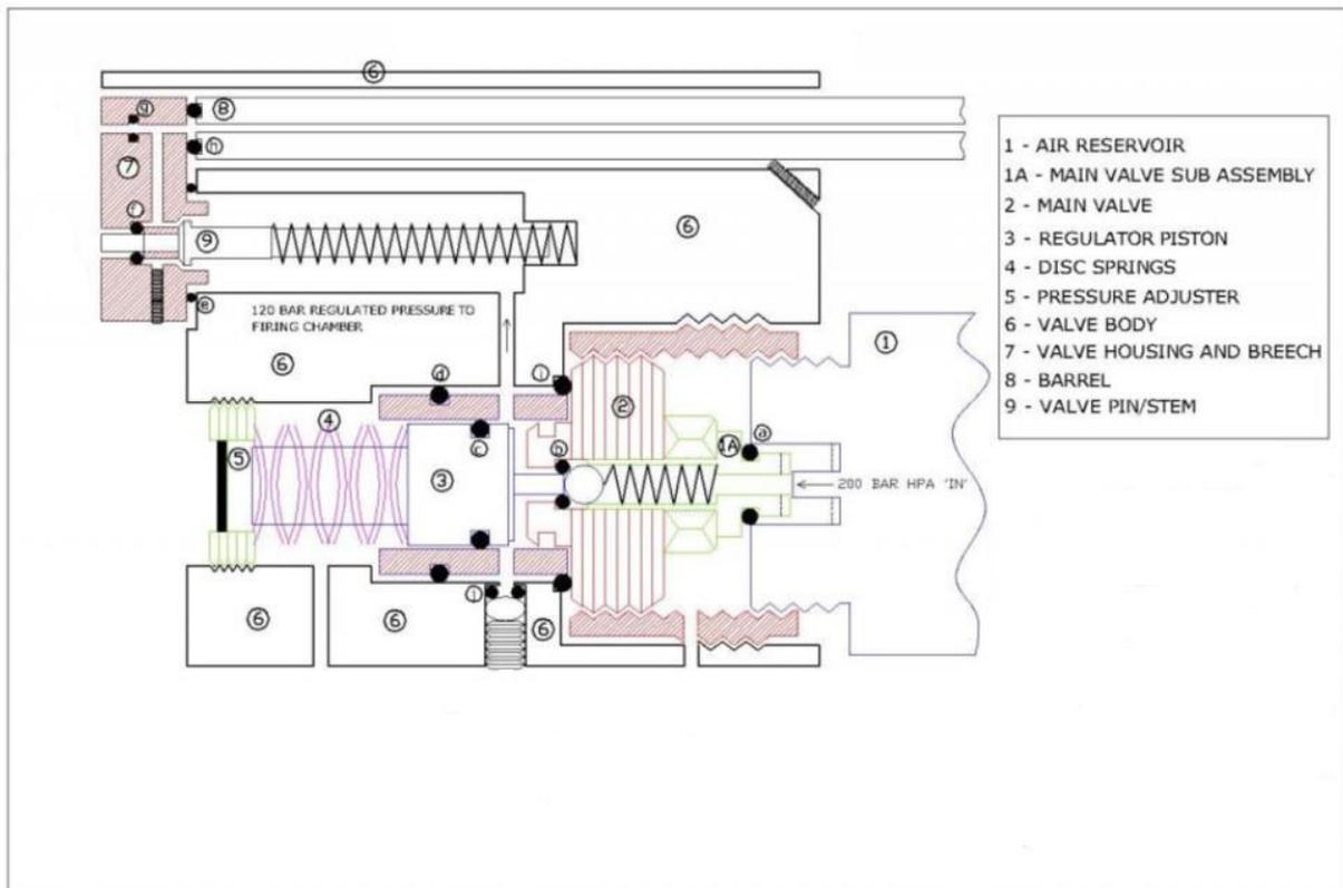
With a fitting socket, unscrew part 1a, to gain access to the ball and spring. Below you see the main valve 2 with main valve subassembly 1a.
