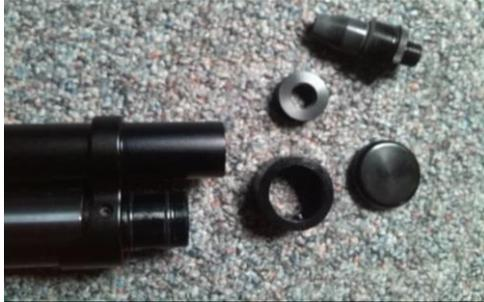
Unscrew the three allen bolts to remove the barrelband
