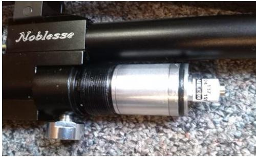
Clean the treads of excessive grease and screw the pressure tube back on the gauge assembly. Leave a gap of about 0,5 mm open between tube and gauge assembly. This gap is needed for proper venting of the regulator.
