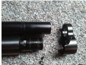
Unscrew the pressure tube. When the tube won't turn loose easy, please check if there is no pressure left in the reservoir!
