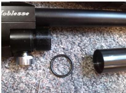
Check the pressure tube if it is free from dirt and scratches where the regulator will come. Also check the pressure gauge adapter if it is clean.
