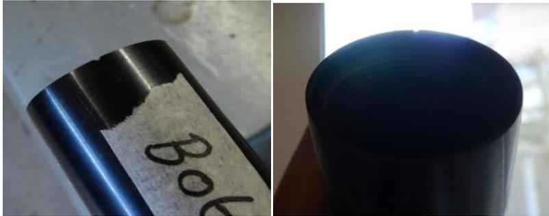
file a small groove in the longitudinal direction of the screw-thread of the valve body. Use the corner of the file to cut a 45 degree/triangular groove in the threads, as shown below,
