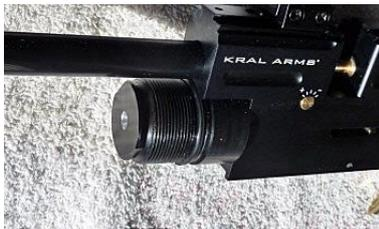
Some valve house come with an double o-ring, one thinner one at the front of the valve house and one larger one on the end of the valve house. Remove both. There are also models with just one o-ring
