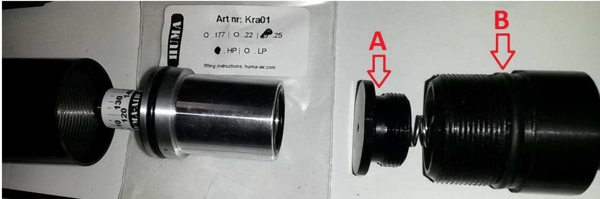
Unscrew the valvehouse cap and place the small o-ring what came with the regulator on the cap "A" Then grease the o-ring seating on the valvehouse a bit for smooth fitting. o-ring "B" has already been removed in the steps before.
