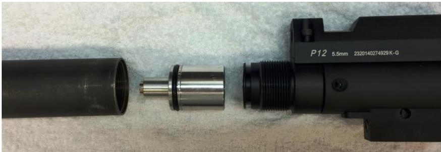
10. Make sure the O-rings are properly seated in the grooves of the regulator
