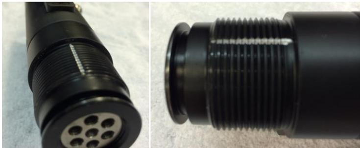
Use the same small metal file to make a tiny notch in the end/edge of the pressure tube. This does not have to be very big/deep, see pictures below. Just a very tiny notch just enough so you can feel it with your fingernail.
