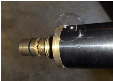
If you are happy that the cylinder is venting as it should then remove the valve body again, and then fit the regulator as described in Method 1,
