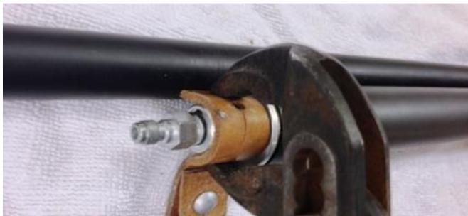
5. You should be able to push the pressure gauge assembly a little forward into the tube, using an allen wrench or wooden dowel that you place in the hole of the pressure gauge.
