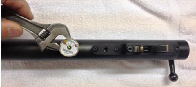
4. Take a pair of pliers to remove the end cap. Use a piece of leather (belt) to prevent damage to the end cap, and unscrew the end cap.
