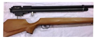
3. Double check / check again if there is absolutely no pressure inside the pressure tube. Only when absolutely certain proceed to remove the pressure gauge.
