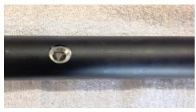
4.Loosen the grub screws from the barrel band and take the barrel band off.
