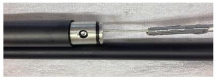
8. You receive your regulator in a small plastic bag. The bag contains the regulator and also a tiny M3 allen flow restrictor bolt that has to be placed inside the adjustment screw. This bolt creates a slower but more accurate regulating behavior.
