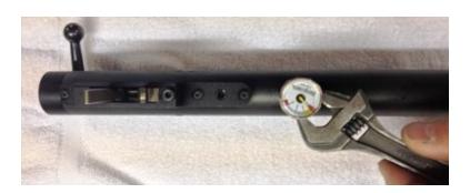
12.On the side of the pressure tube near the breech and valve you will find the factory flow restrictor that restricts the airflow through the valve house. There are 2 grub screws on top of each other.
